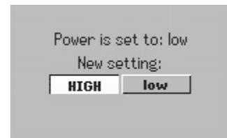
Switching the Power to the high setting means that the drain on the batteries increases about 10 to 15% and the signal strength will increase by about 10dB. Upon exit of UI Messenger, the software will return this setting to low.
